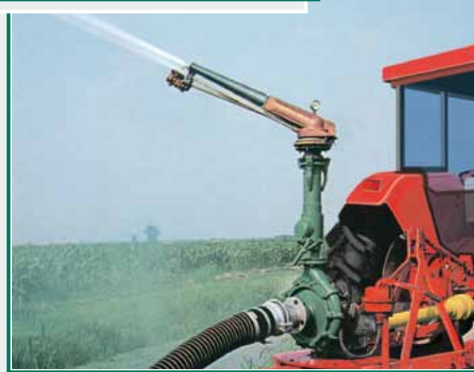
Applicazione al sollevatore del trattore Tractor hydraulic lift mounted pump outfit Emploi sur relevage du tracteur
